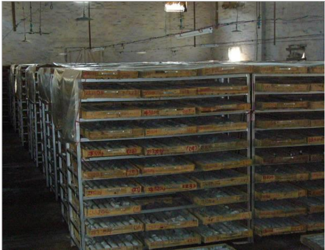
a) Drill core racks in core shack
