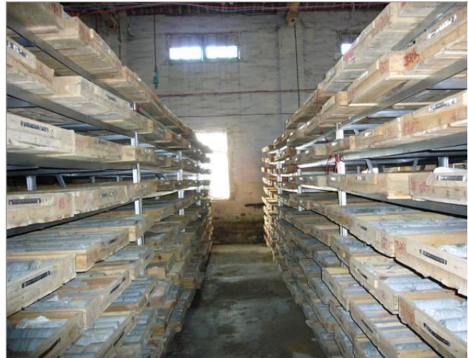
b) Drill core racks in core shack
